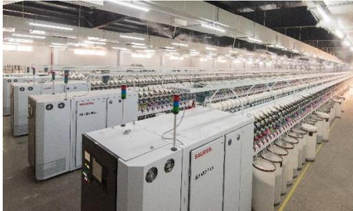
The BD 480 Plus semi-automatic rotor-spinning can be customised according to customer requirements, with a maximum machine length of up to 512 spinning positions.
